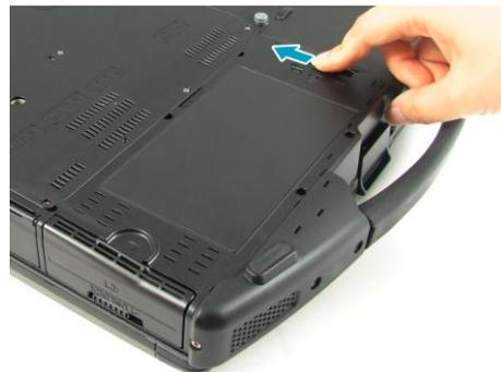
2. Slide the battery latch to the right (as shown in the illustration) and hold it in place. Then pull the battery out to disengage it from its compartment.
