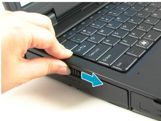
2. Press Eject button to eject the tray.
