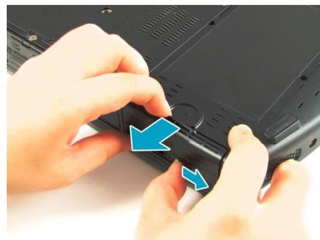
3. Remove the battery out of the battery compartment.
