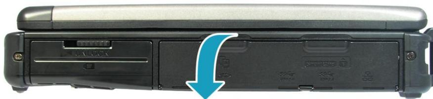
2. Insert a smart card into the smart card slot.
