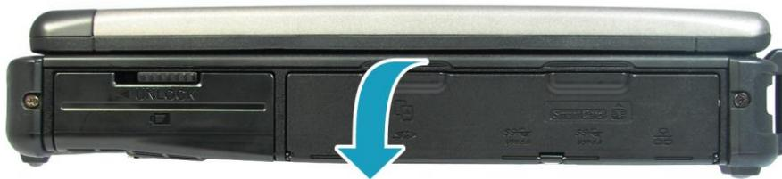
2. With the label side down, push the memory card into the memory card slot until it clicks into place.
