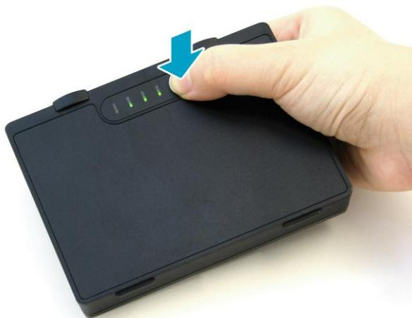
The remaining battery power is indicated by the four **Green** LEDs.
