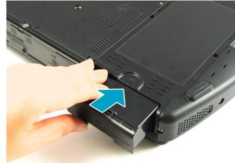
3. Slide the battery latch to the lock position to secure the battery.
