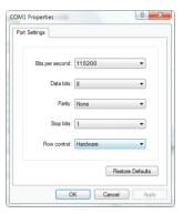
You can see the setting parameters of serial port from self-test page, Click "Apply", then click "OK" (Note: This setting must consistent with the setting parameters of serial port from the printer self-test page, otherwise it will be garbled case) appears as shown below:
