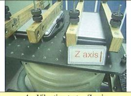
Vibration test -- Z axis
