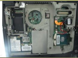
10. Appearance of the interior of specimen after waterproof test
