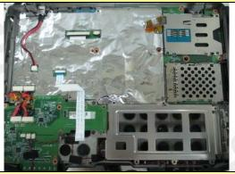
Appearance of the interior of specimen after waterproof test
