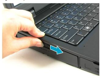
2. Press Eject button to eject the tray.
