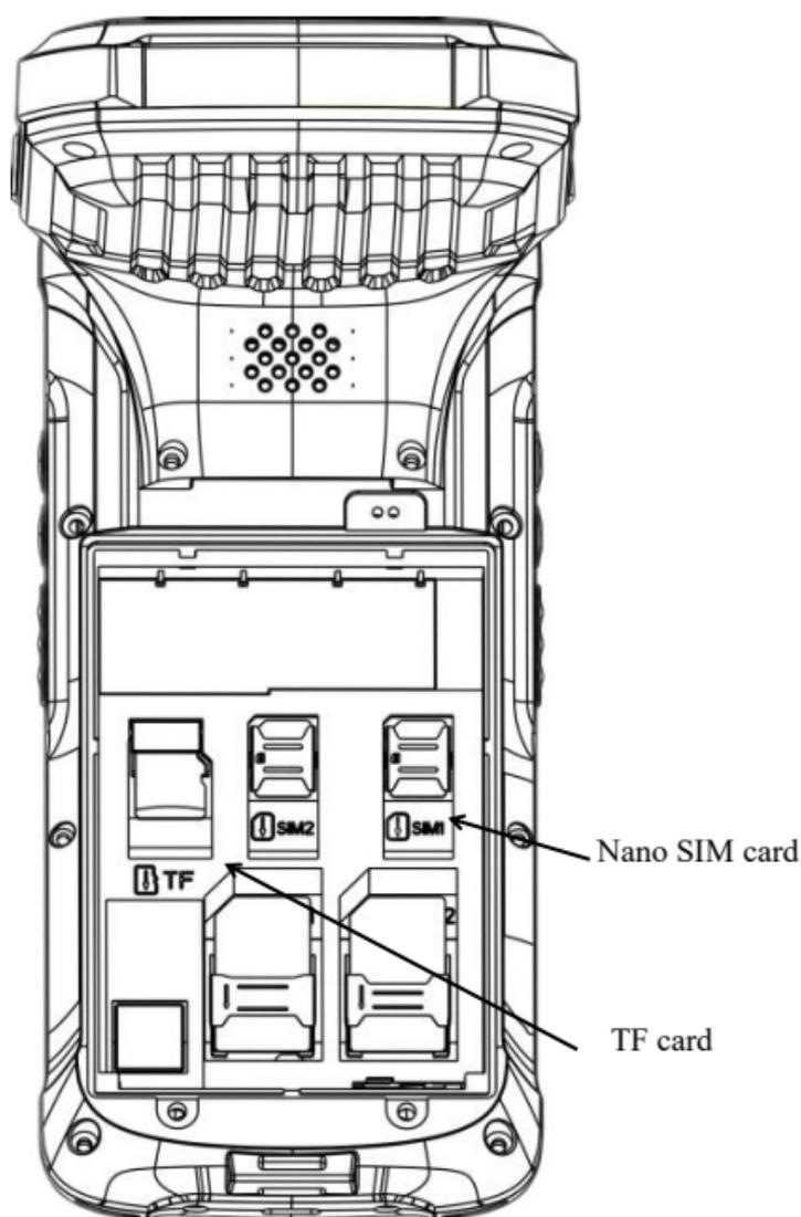
(Warm tips: The handheld terminal only supports Nano SIM card, standard SIM card slot is for PSAM card)
