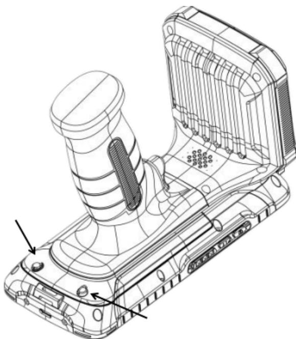
2. Remove the battery cover and battery in the direction of the arrow.
