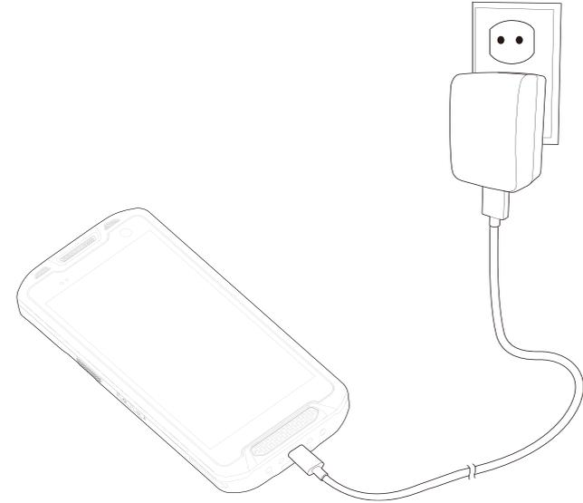
1. Assemble the AC plug, power adapter and USB cable.
