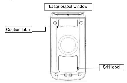
If the above laser light label is attached to your device, it indicates the product contains a laser engine or laser aimer that emits the laser light. The following information is provided to comply with the rules imposed by international authorities and refers to the correct use of PM3 Bluetooth scanner.
