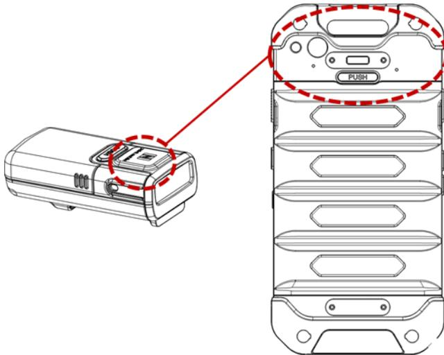
Figure 33 Tap-to-Pair\_Align PM5 and PM85
