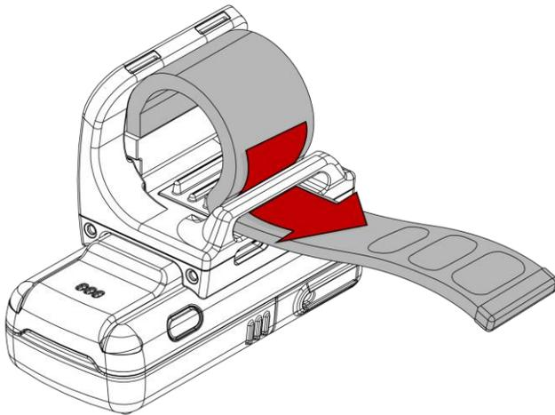
2. Wear the PM5 with single trigger on the index finger as the trigger scan button facing the thumb.
