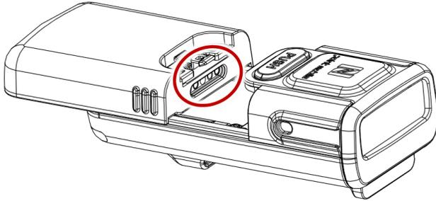
2. Slide and press the battery into the battery slot so that the battery is firmly engaged
