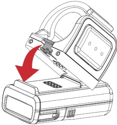
Figure 11 Trigger Assemble\_Right hand mount
